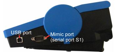
The Mimic port is the second port from the front, on the right-hand side of the MB-LS, and it is the larger of the two ports. You can feel the pins. You can connect either end of the cable to the MB-LS; it is reversible. The connector will only go in one way.
