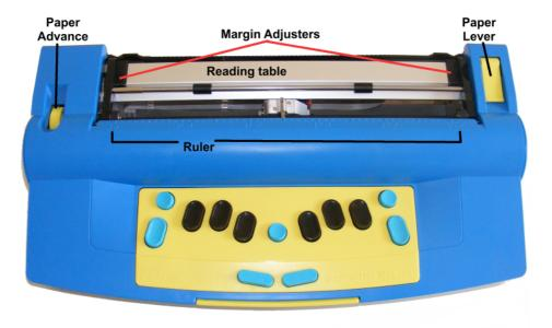
Illustration 5: The top of the MB-LS, cover off, with the Embossing Area labelled right place for your Braille.
