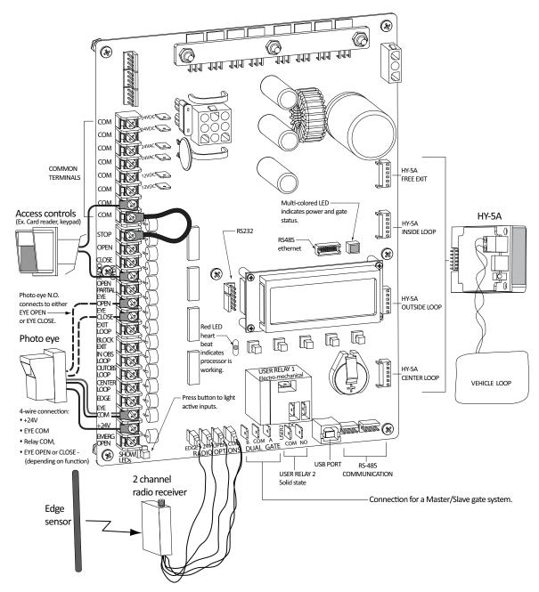
Figure 4-5. Entrapment Sensor Connections
