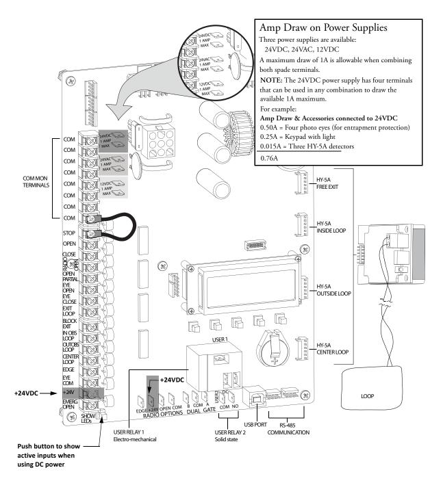
Figure 4-2. Smart DC Controller Board
