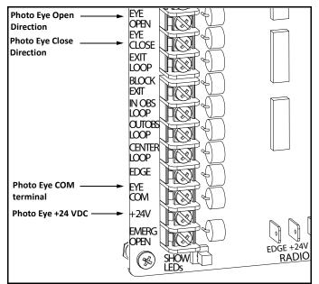
Figure 6-9. Connections for Entrapment Protection only
