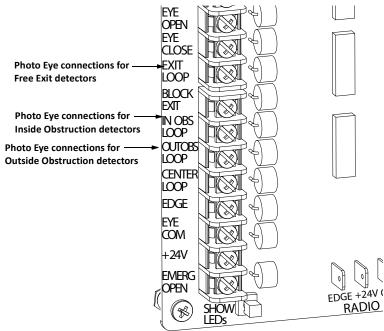
Figure 6-10. Connections for Loop Detectors
