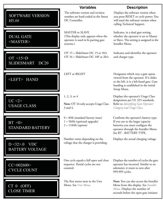
Figure 3-6. Operator Status Displays
