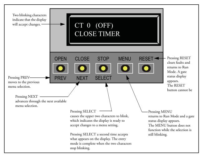
Figure 3-3. Function of the Smart DC Controller Buttons in Menu Mode
