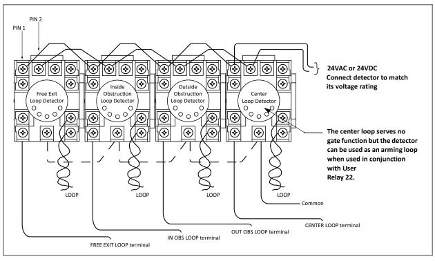
Figure 4-4. Standard 11-Pin Box Type Vehicle Detector
