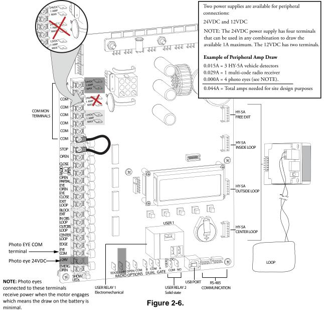
To connect any peripheral devices to a solar operator, use the 24VDC or 12VDC terminals. Because a solar operator gets its energy from the sun and stores the energy produced by the solar panels in batteries that are constantly discharging, it is important to use peripheral devices that draw and consume as little power as possible.
