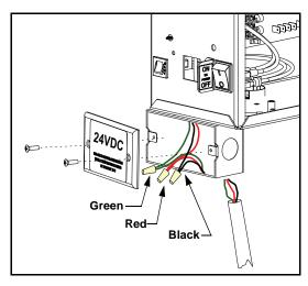
Figure 2-4. Solar Panels and Wiring Connections
