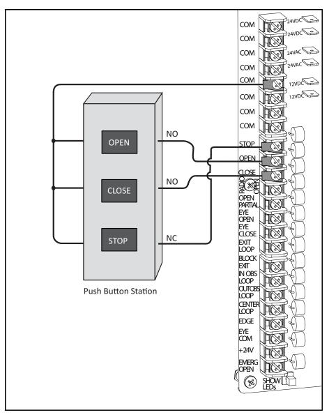
Figure 4-6. Manual Push Button Station Connection
