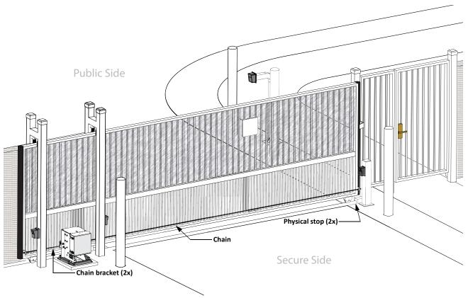
**Note:** Several different ways to mount the SlideSmart operator exist. A few are shown here. For more detailed drawings, refer to the Installation Configurations in the Appendix.
