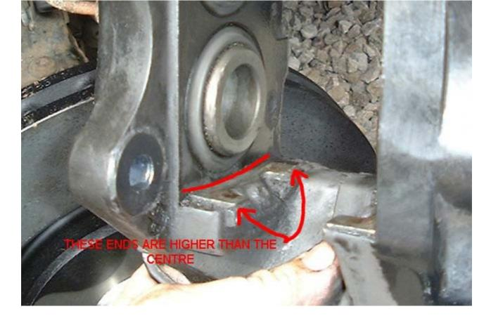
This is a good time to push the four pistons back into the caliper to aid fitting later.Undo the bleed nipple which will release a bit of fluid but it will make pushing back the pistons easier. Tighten the bleed nipple when the pistons are flush with the caliper.
