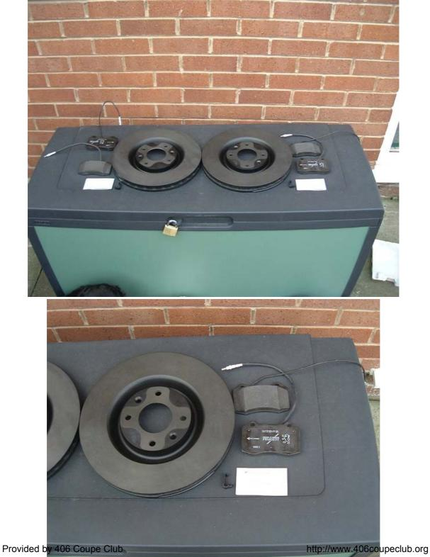
One pair of Brembo front discs (305mm diameter), One set of OEM Pads which include 2 sachets of grease & 2 new pipe clips (Part No - 425251)
