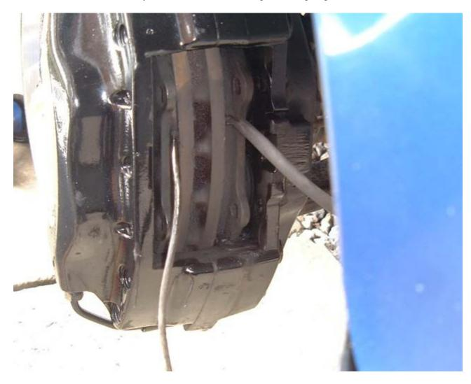
You now need to pull the worn pads out of the caliper. This can be tricky because of the rim that is worn on the edge of the brake disc. I used a screwdriver like in the picture below to prise the pads away from the discs and force the pistons into the caliper which enabled the outside pad to freely pull out. The inside pad was still stuck in the caliper, even when I had pushed the piston back in, caused by a problem I found later.
