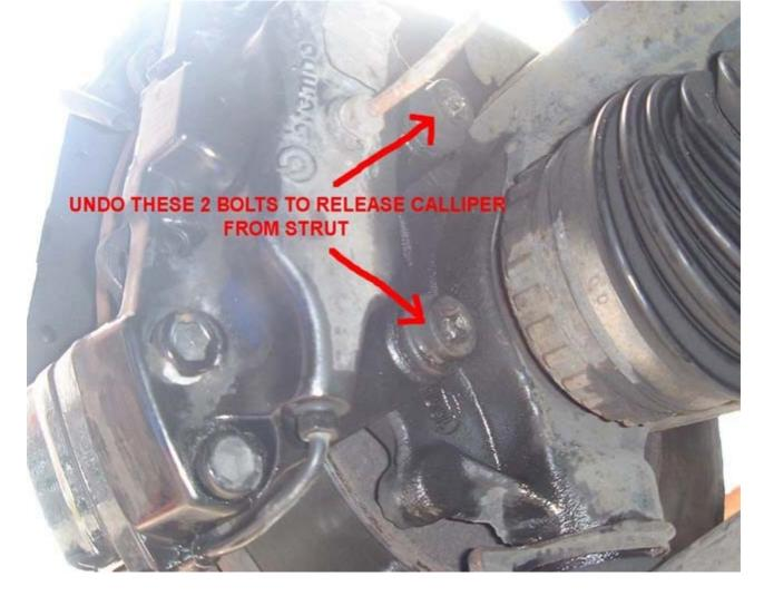
When you have eventually undone the bolts the caliper will come away from the disc. Pull up the tab shown below to release the brake pipe from the strut.
