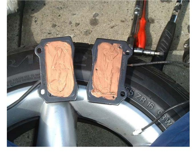
Note on the pads that one pad has a thin wear indicator cable and the other has a thicker cable. On mine, the pad with the thicker cable went to the side nearest the car(inside) and the other obviously to the outside. You�ll also notice that the cables are not on centre of the pad lengthways, and the pads need to go in the caliper with the cables to the top.(I only noticed this after I greased the pads up, that�s why the picture above shows an odd pair).
