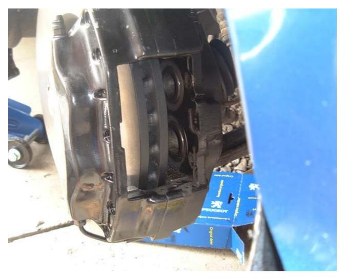
Before fitting the pads, apply the copper grease supplied to the back of the pads ensuring non gets on the pad itself.
