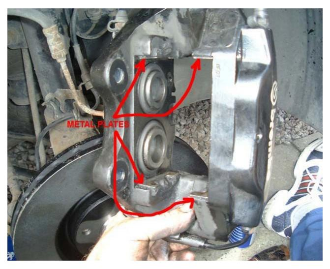
The next picture shows the bottom inside plate and you can just see the curvature of it.
