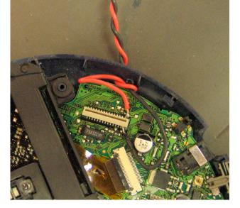
multi-meter to locate an acceptable place to hack into the play button (+) and (-). Drill a hole through the CD player casing to run 24-gauge stranded wire through. Use hot glue to secure the wires in place before soldering. (Unsecured wires will rip the circuitry loose from the circuit)
